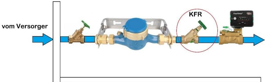
Fig. 10.2.2: KFR valve water meter
